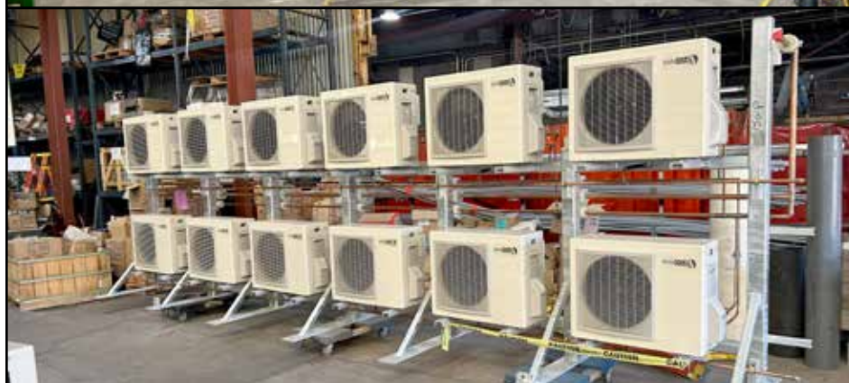
Pictured top is one of many domestic hot water prefabricated skids constructed at signatory contractor Broadway Mechanical's shop. Pictured below are banks of heat pumps designed and fabricated in their shop, ready to be sent out.
